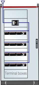
ArTu L Series dim.1600x800x195 (1750x890x240)mm (external hxwxd) IP43 complete with internal cable container w=200mm, plate for Tmax T3-XT3, and modular panels
