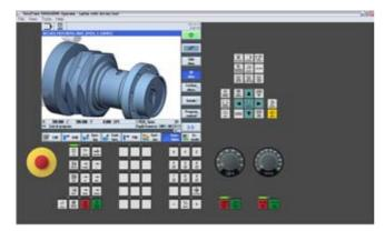
SinuTrain for SINUMERIK Operate is a PC-based CNC training/ CNC programming software package. SinuTrain for SINUMERIK Operate enables completely identical operator control and CNC programming as on SINUMERIK CNC systems that are equipped with graphical user interface SINUMERIK Operate.
