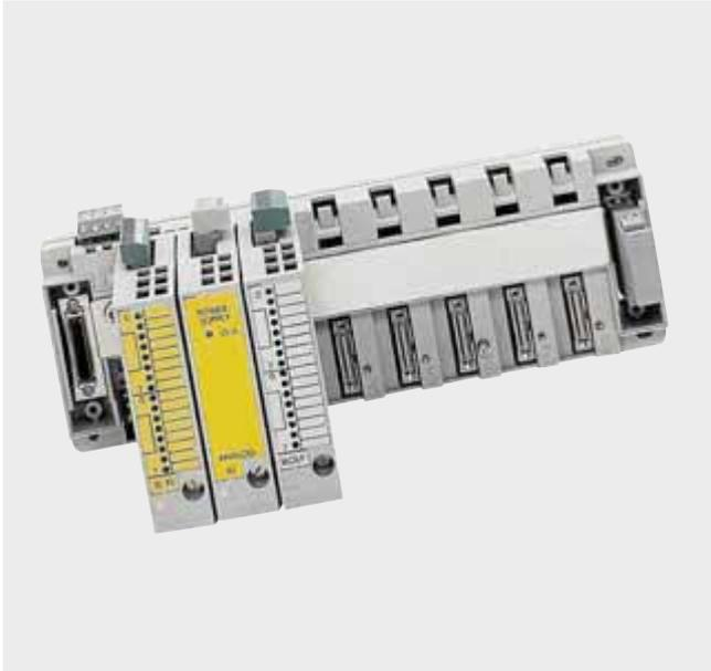
For rapid movement synchronization and/or for safety-oriented input/output signals on the NCK channel of the SINUMERIK Safety Integrated<sup>1)</sup> safety function, digital and analog CNC inputs/outputs can be connected to the drive bus via the NCU terminal block (max. 2) when using the SINUMERIK 810D powerline and SINUMERIK 840D powerline.
