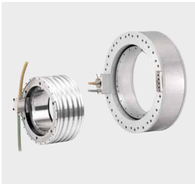
1FW6 built-in torque motors are liquid-cooled, multi-pole permanent-magnet AC synchronous motors with hollow-shaft rotor. The 1FW6 motors are supplied as built-in components that are held together in the delivered state by transport locks. For a complete drive unit, an additional bearing and shaft encoder are required.
