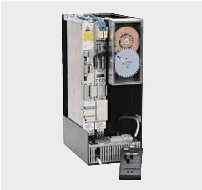
The training case can be used for customer presentations and for teaching technical aspects of configuration, start-up and service. With the Motion Control variant, functions such as synchronous operation or positioning can be simulated using the toothed discs with scale divisions and stroboscopic equipment.
