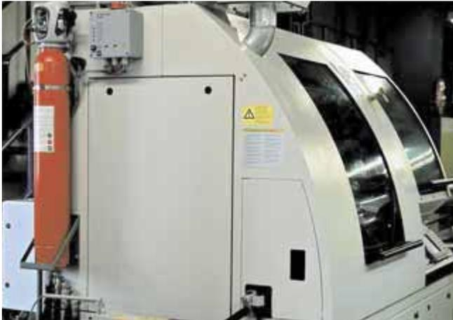
Sinorix al-deco are automatic fire-extinguishing systems for machine tools. Sinorix al-deco fights the fire where it breaks out – in the machine tool – without posing a risk to people, the environment, or technical components.
