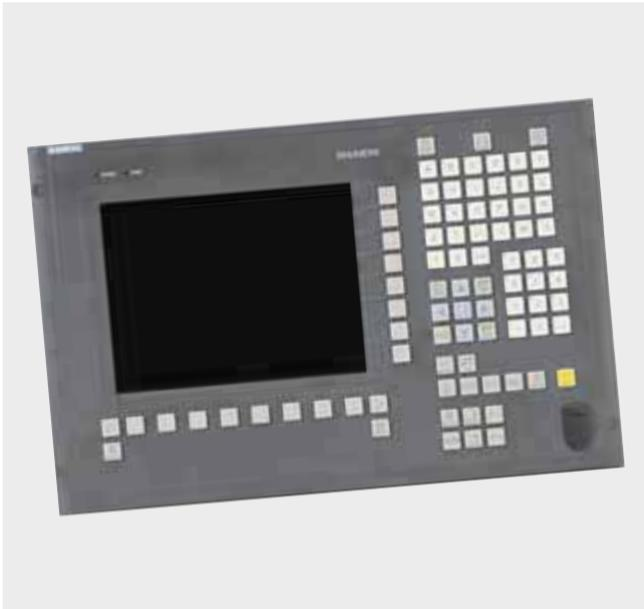
The SINUMERIK OP 010C operator panel front with 10.4" TFT color display with a resolution of 640 x 480 pixels (VGA) features a 65-key mechanical keypad with 8 + 4 horizontal and 8 vertical softkeys.
