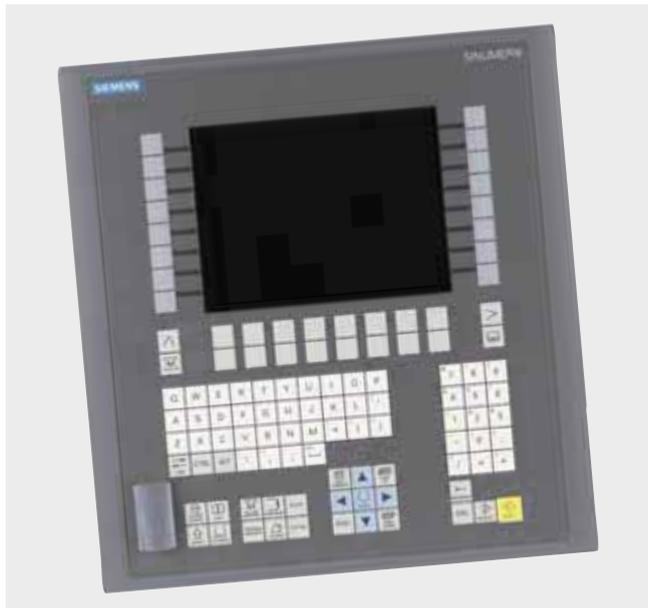
The extremely compact SINUMERIK OP 08T operator panel front supports the distributed installation of the operator panel front and control. The SINUMERIK OP 08T operator panel front contains a membrane keyboard with 65 keys (layout as SINUMERIK KB 310C full CNC keyboard), as well as 2 x (8 + 2) horizontal and 2 x 8 vertical softkeys.
