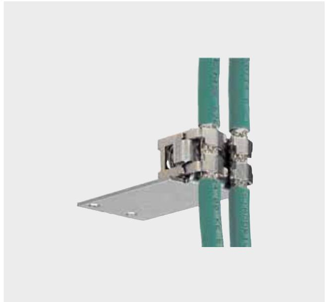
The shield connection is used for contacting the signal cables of the closed-loop control to the module housing's frame potential in accordance with the EMC Directive. The shield connection is available for 2 or 4 cables.
