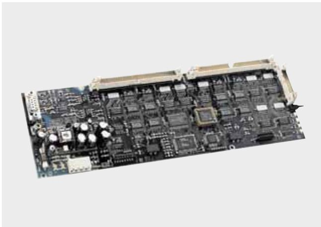
Customers can connect their own operator panels using the SINUMERIK MPI interface. The unit provides digital inputs and outputs, and an MPI communications interface for this purpose.
