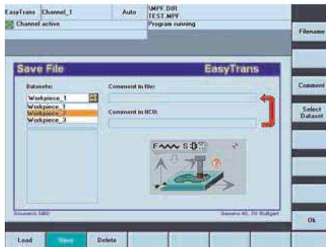
EasyTrans is a simple tool for administration of data blocks. Various parameter areas (R parameters, PLC data blocks and PLC bit memories) can be saved in a backup file on the HMI, and downloaded back into the control. EasyTrans can create, read and delete several backup files in a directory. It is configured using entries in an INI file.
