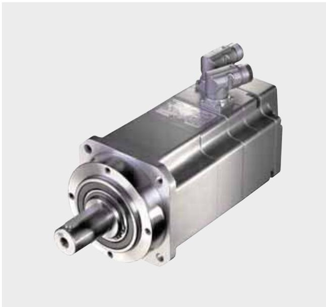
The 1FK7-DYA compact geared motor combines electrical and mechanical components in the smallest space possible. This mechatronic unit consists of a permanent-magnet 1FK7 synchronous motor and a directly mounted single-stage planetary gearbox.
