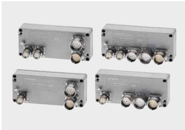
The SME91/SME92/SME93/SME94 encoder connection boxes enable motor and position encoder sensors to be connected in the vicinity of the motor in the case of drives with built-in motors. The encoder connection box is responsible for protecting the motor and outputting the current operating temperature/over-temperature to the converter system without time delay.
