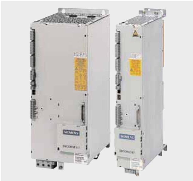
The infeed modules (UI - unregulated, I/R - infeed/regenerative feedback module, regulated) are connected to TN line supplies 380 V<sup>1)</sup>/400 V/415 V 3 AC ± 10 %; 480 V + 6 %/- 10 %; 50/60 Hz. The infeed modules generate the DC link voltage for the drive group and the voltages for the electronics. The voltages for the electronics centrally supply the drive modules and the modules of the SINUMERIK 810D powerline/840D powerline – possibly included in the group – via the device bus.
