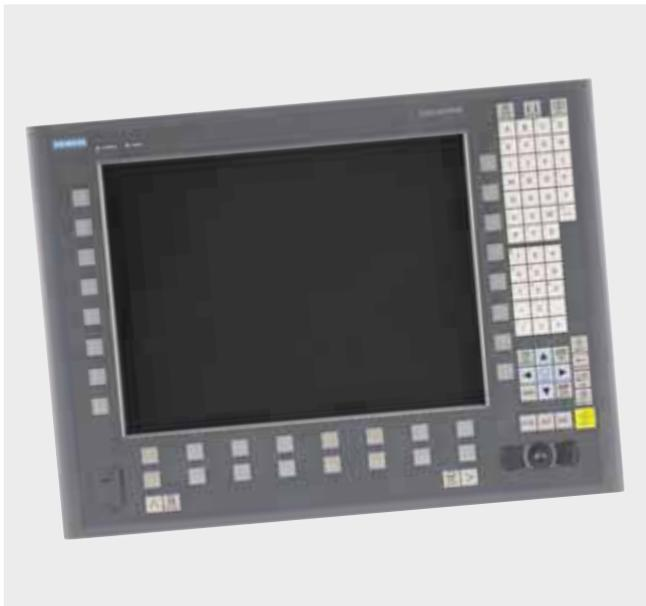
The SINUMERIK TP 015AT touch operator panel front with 15" TFT color display, 1024 x 768 pixels (XGA) and touch screen supports the distributed installation of the operator panel front and control. The SINUMERIK TP 015AT touch operator panel front contains a membrane keyboard with 62 keys as well as 2 x (8 + 2) horizontal and 2 x 8 vertical softkeys and an integral mouse.
