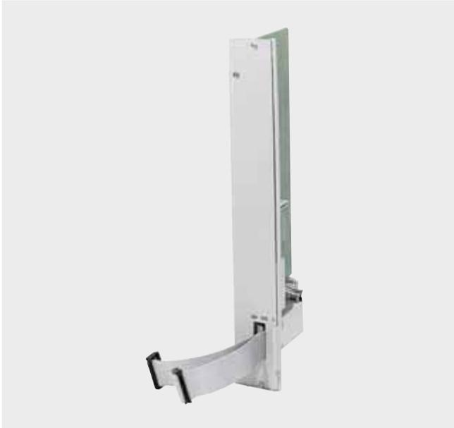
To expand the SINUMERIK 810D powerline to up to 6 axes, axis expansion plug-in units are required. These are inserted in the power modules of the SIMODRIVE 611 digital, where they take the place of the closed-loop control plug-in units.
