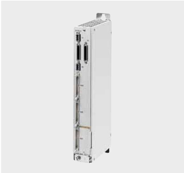
The single I/O module EFP has 64 inputs and 32 short-circuit-proof outputs. The total current for the outputs is 12 A, i.e. 32 outputs with 0.5 A each and a simultaneity factor of 0.75.
