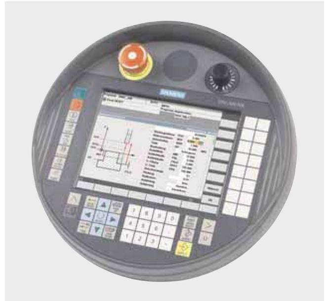
The mobile SINUMERIK HT 8 handheld terminal combines the functions of an operator panel and a machine control panel in a single device, permitting complete operator control and monitoring of machines. It can be used as a supplementary main operator panel or as a secondary control panel. The safety system is designed to allow personnel to work in the machine's hazard zone.
