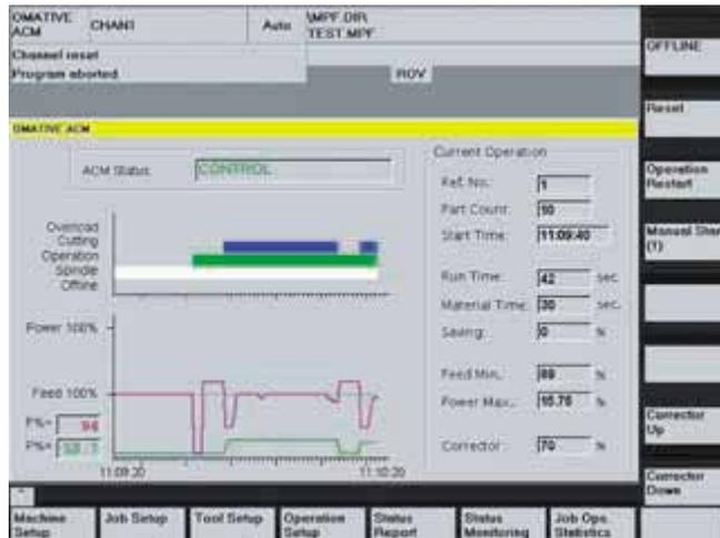
**ADAPTIVE CONTROL & MONITORING (ACM) for real-time feedrate optimization**
