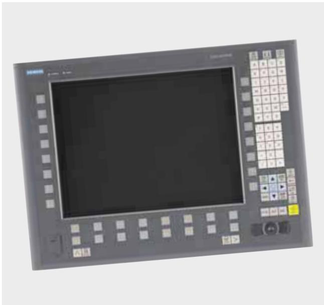
The SINUMERIK OP 015AT operator panel front with 15" TFT color display, 1024 x 768 pixels (XGA), supports the distributed installation of the operator panel front and control. The SINUMERIK OP 015AT operator panel front contains a membrane keyboard with 62 keys as well as 2 x (8 + 2) horizontal and 2 x 8 vertical softkeys and an integral mouse.
