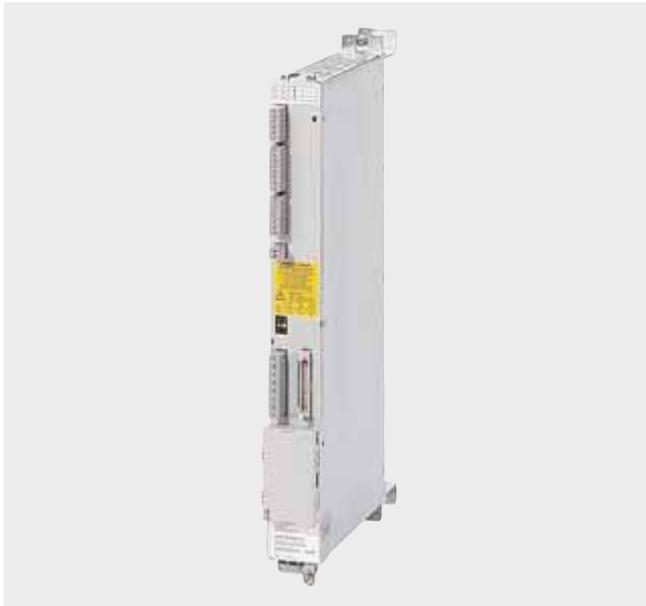
The monitoring module is used to expand the electronics power supply if in a group a higher number of drive modules require a higher electronics power supply rating. The monitoring module includes central monitoring functions for a separate drive group. The monitoring module power supply can be taken from a 380 V to 480 V 3 AC line supply as well as from the DC link voltage – or from both e.g. for the ESR function (emergency retraction).
