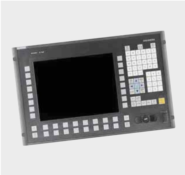
The SINUMERIK OP 012 operator panel front with 12.1" TFT color display with a resolution of 800 x 600 pixels (SVGA) features a 59-key membrane keypad as well as 2 x (8 + 2) horizontal and 2 x 8 vertical softkeys. The integral mouse provides an additional method of machine control. The 2 x 8 vertical softkeys can be used as direct keys.
