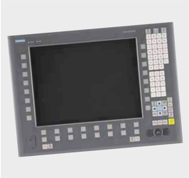
The SINUMERIK TP 015A touch operator panel front with 15" TFT color display with a resolution of 1024 x 768 pixels (XGA) and touch screen features a 62-key membrane keyboard, as well as 2 x (8 + 2) horizontal and 2 x 8 vertical softkeys and an integral mouse. The 2 x 8 vertical softkeys can be used as direct keys in the PLC.
