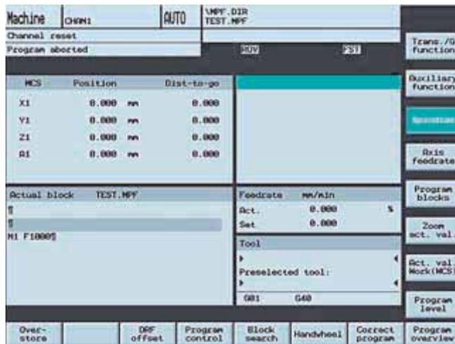
The HMI-Embedded software is a technology-independent, multi-channel operating software for machine tools and executes on an embedded operating system. The software supports convenient and complete window-oriented operation of machines.
