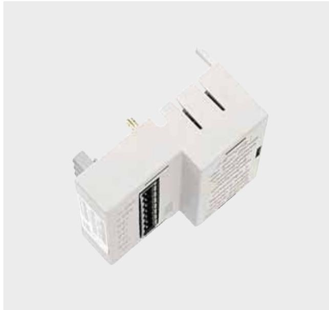
The overvoltage limiter module limits transient overvoltages that occur as the result of, for example, switching operations on inductive loads in the line supply to acceptable values. For 10 kW infeed modules and higher, this overvoltage limiter module is plugged into the X181 interface.
