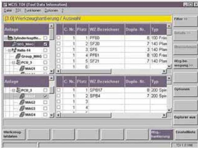
Using the convenient dialog prompting of TDI Toolhandling, you can import, buffer or forward tool data when loading and unloading – over the network. Any containers within a plant can be involved in the processes. The objective is to obtain a closed tool data circuit.
