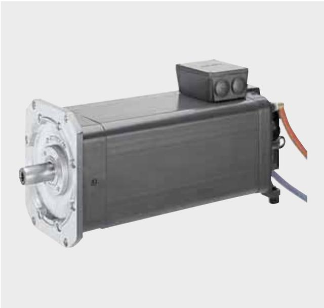
Given the compact design of modern machines, the heat loss from electrical drives can have an adverse effect on the accuracy of machining. The resulting demands for cold motors with a high power density led to the development of the water-cooled 1PH4 motors.
