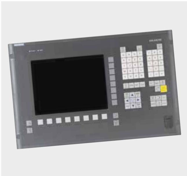
The SINUMERIK OP 010 operator panel front with 10.4" TFT color display with a resolution of 640 x 480 pixels (VGA) features a 62-key membrane keypad with 8 + 4 horizontal and 8 vertical softkeys that has been optimized for programming subroutines.
