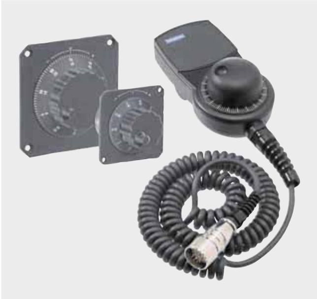
This encoder generates signals which correspond to the movements of the handwheel as it is turned. The axis selected via the control can be positioned paraxially. The handwheels are equipped with a magnetic latching mechanism that supports traversing with incremental accuracy.
