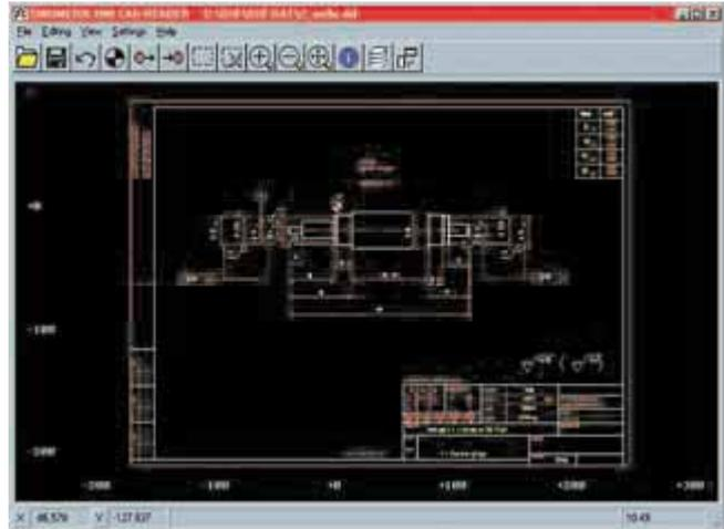
The CAD Reader program converts DXF files into contours or hole drilling templates.
