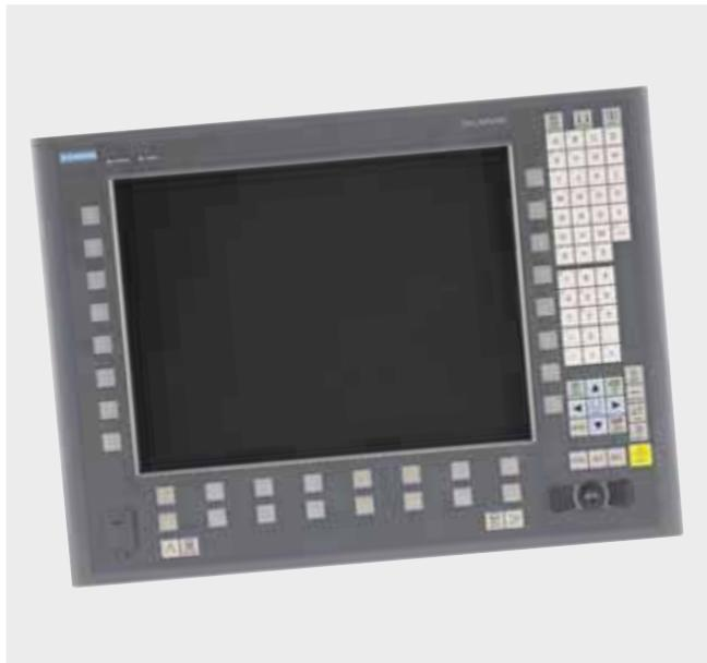
The SINUMERIK OP 015A operator panel front with 15" TFT color display with a resolution of 1024 x 768 pixels (XGA) features a 62-key membrane keyboard with 2 x (8 + 2) horizontal and 2 x 8 vertical softkeys and an integral mouse. The 2 x 8 vertical softkeys can be used as direct keys in the PLC.
