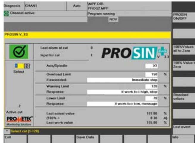
PROSIN PLUS tool monitoring as integrated software solution for the SINUMERIK 840D sl control
