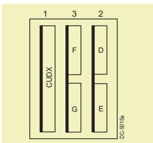
Position of mounting slots 1 to 3 and slots D to G in the electronics box
