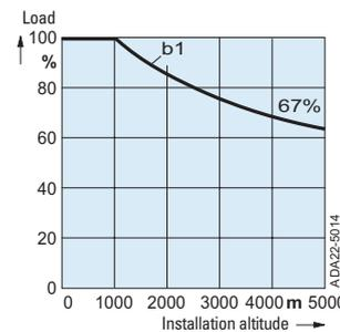
Curve b1: Reduction factor of load values (DC current) at installation altitudes above 1000 m.
